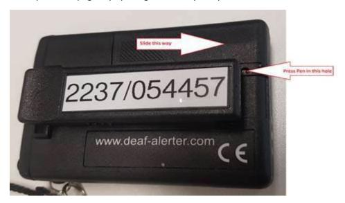
Close the battery compartment by sliding the hatch closed. The pager should vibrate when powered up and the liquid crystal display will provide the pagers unique identifying details. When this happens, the pager is ready for use. Once tested please remove the battery from the pager as outlined above and return both to the brown envelope in the building fire folder.
